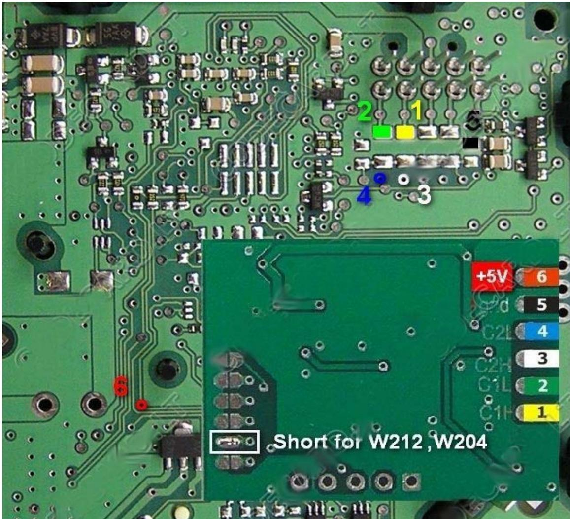
Remove from EZS board SMD part marked with red "X". With short, good isolated wire connect Mercedes CAN filter to EZS board according picture: 1-1 (C1H), 2-2(C1L), 3-3(C2H), 4-4(C2L), 5-5(GND), and 6-6 (+5V).
