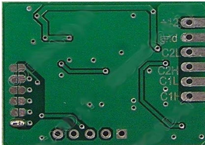
Remove from EZS board SMD part marked with red "X". With short, good isolated wire connect Mercedes CAN filter to EZS board according picture: 1-1 (C1H), 2-2(C1L), 3-3(C2H), 4-4(C2L), 5-5(GND), and 6-6 (+5V).
